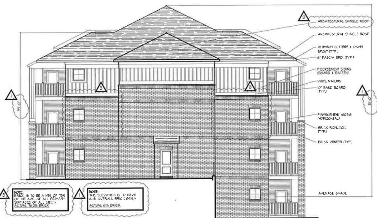
BUILDING B- RIGHT SIDE ELEVATION
