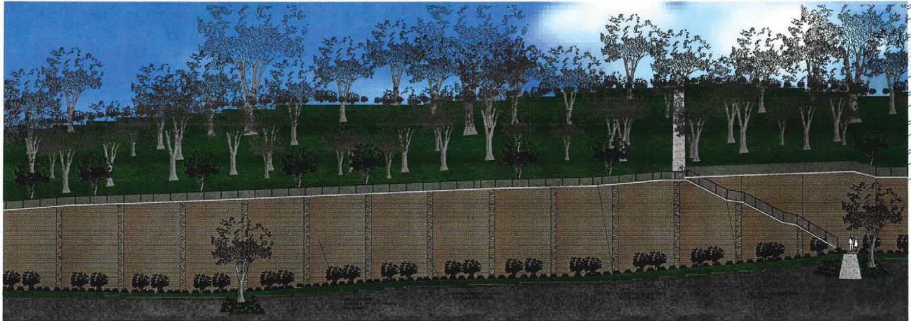
PARTIAL ELEVATION OF SOIL NAIL RETAINING WALL
