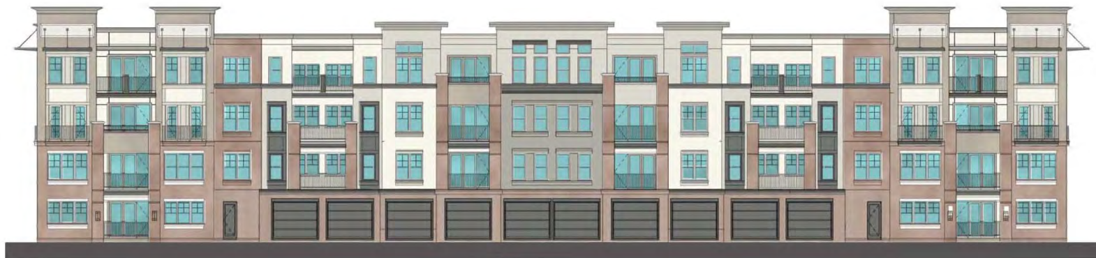
BUILDING TYPE A - REAR ELEVATION BUILDING HEIGHT 49' - 1"
