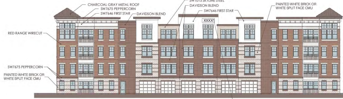
C2 BUILDING TYPE B - REAR ELEVATION 332' = 1'-0"
