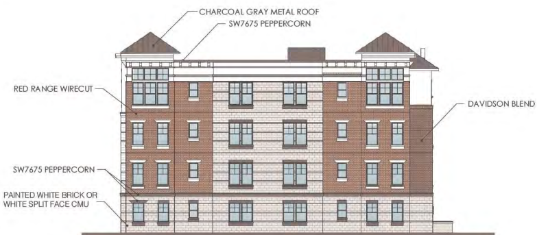
H6 BUILDING TYPE B - RIGHT SIDE ELEVATION 332' = 1'-0"
