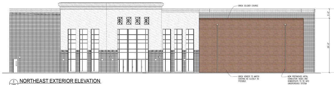
2 NORTHEAST EXTERIOR ELEVATION 1/8"=1'-0"
