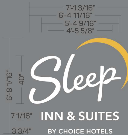
CHANNEL LETTER DETAIL SCALE: 1/4" = 1'-0"
