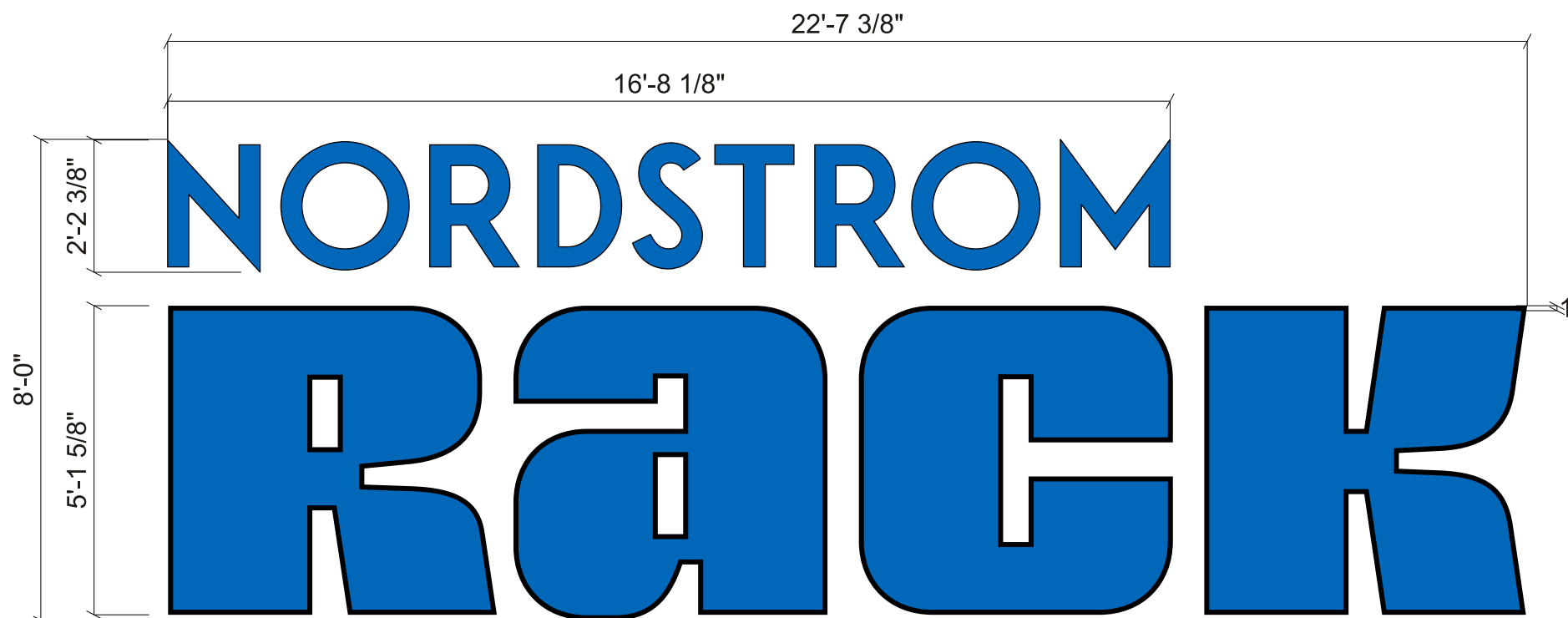
A FRONT VIEW @ FACE LIT REVERSE CHANNEL LETTERS Scale: 3/8"=1'-0"
