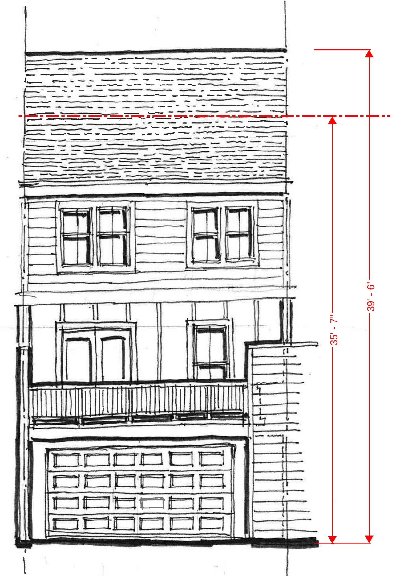
REAR ELEVATION THREE STORY TYPICAL
